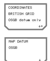
The unit stores the positions it calculates (and the waypoints you enter) in the WGS84 datum and as height above ellipsoid (HAE). A position is converted from WGS84 and HAE to the systems you have selected when it is displayed. Since Lat/Lon and UTM are global systems, they can be used to describe locations anywhere on earth. A position in the area described by British grid can therefore be described in Lat/Lon, UTM, or British grid. It cannot be described in UPS or Irish grid.
