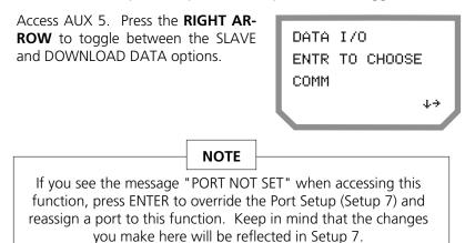
Select "COMM" to use the COMM module of the PPSW to download data files, almanac, routes and waypoints, grids, datums, setup parameters, or attributes from the receiver to a PC as well as uploading almanacs, routes and waypoints, setup, grids, datums, and attributes from a PC to the receiver. Select DOWNLOAD DATA to download real-time data, almanac, ephemeris, waypoints, averaged position, or the POS data buffer to a PC from the receiver using the LOG software.
