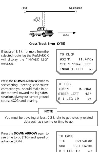
Time to go (TTG), on the second line of the screen above, is the length of time required to complete the current leg, given the current speed of advance.
