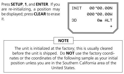
To select position coordinates, press the appropriate keys on the 10-key keypad. You may have to select a hemisphere; the unit automatically displays "N" during initialization. If your position is south of the equator, press the **RIGHT ARROW** to select "S." Next, press **ENTER**.
