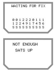
The unit devotes all ten channels to the search for the satellite the almanac indicates is directly overhead, given your last fix or initial position. This generally takes a few seconds. If the satellite cannot be located, the unit looks for the satellite with the next highest elevation. Searching for the highest satellite greatly shortens the length of time required to obtain a position fix.
